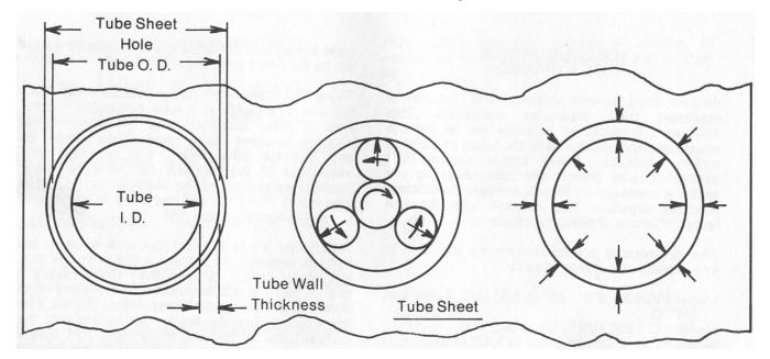
Step A - Measure Tube Sheet Hole
